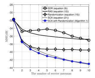
**Figure 6.** MSE performance of the proposed MIMO AirComp framework and other receive beamforming techniques, when SNR is 10 dB, objective function is arithmetic mean, and  $N_T = 2$ , K = 20.
