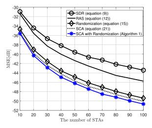
**Figure 5.** MSE performance of the proposed MIMO AirComp framework and other receive beamforming techniques, when SNR is 10 dB, objective function is arithmetic mean, and  $N_T = 2$ ,  $N_R = 4$ .
