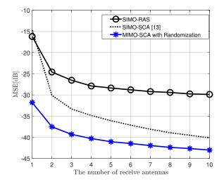
**Figure 3.** MSE performance of the proposed MIMO AirComp framework and conventional SIMO AirComp, when SNR is 10 dB, objective function is arithmetic mean, and  $N_T = 2$  (in MIMO AirComp), K = 20.
