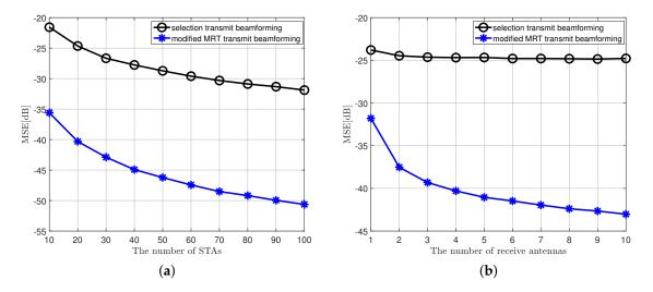
**Figure 4.** MSE performance of the proposed MIMO AirComp framework and other transmit beamforming technique, when SNR is 10 dB, objective function is arithmetic mean. (a) MSE performance when  $N_T = 2$ ,  $N_R = 4$ . (b) MSE performance when  $N_T = 2$ , K = 20.
