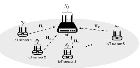
**Figure 1.** System model of the uplink multiple-input multiple-output (MIMO) wireless internet-of-things (IoT) sensor network.
