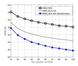
**Figure 2.** Mean squared error (MSE) performance of the proposed MIMO over-the-air computation (AirComp) framework and conventional single-input multiple-output (SIMO) AirComp, when signal-to-noise ratio (SNR) is 10 dB, objective function is arithmetic mean, and  $N_T = 2$  (in MIMO AirComp),  $N_R = 4$ .
